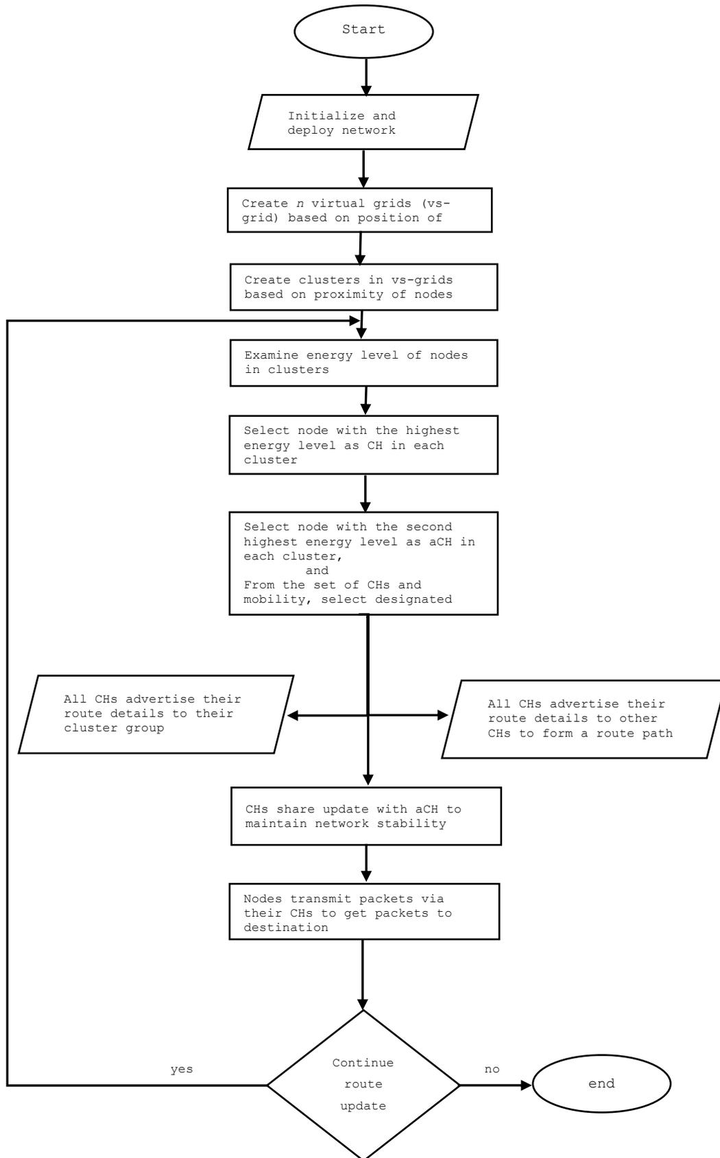
**Figure 4. Flowchart for the creation of virtual grids and clusters; and selection of CHs, aCHs and dCHs selection.** The deployment of nodes and the creation of virtual grids and clusters is shown in Figure 4. At the start of the flowchart, the deployed nodes are initialised. This is followed by the
